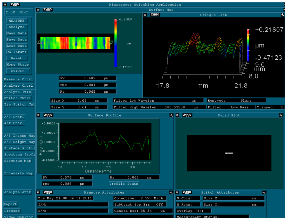
Figure 4-11 Low Pass Waviness: 4mmx1mm Un-Polished Wafer
